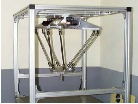
Figure 3. A haptic VR system with parallel active handle: experimental
